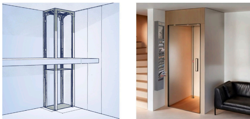
FIGURE 2 | Construction of the vertical lift system as a model (left) and a visualization in the home environment (right). (Rapid review, Switzerland, 2014–2024).
